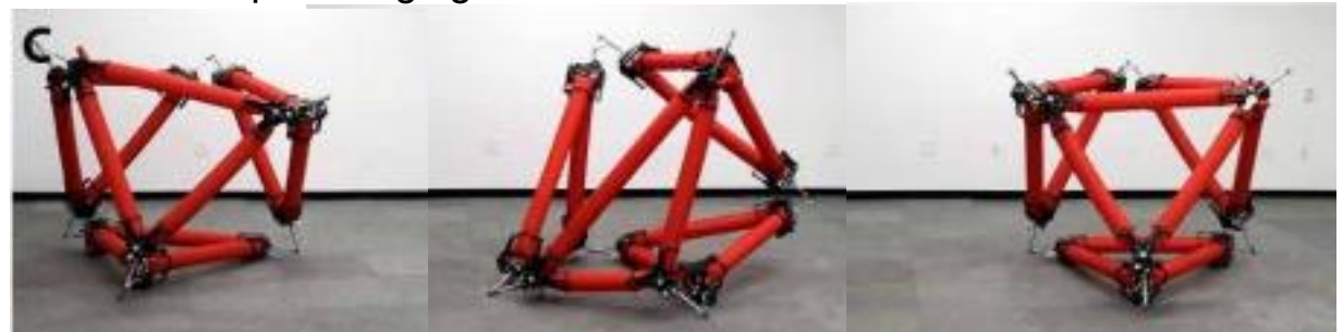
Inflatable shape changing trusses
